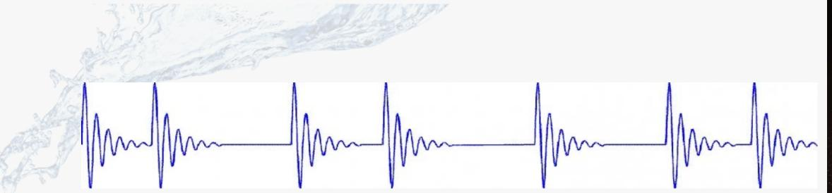
These highly efficient, non-intrusive electronic descalers are installed directly on the water pipe seamlessly integrating into your existing plumbing system. HydroFlow works by emitting a robust yet harmless 150kHz signal throughout the system—whether it's copper, PEX, or PVC—triggering a natural process within the water.
